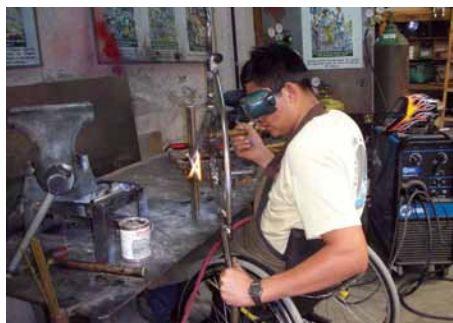
Efrain welds a custom wheelchair frame—the workshop will produce 200 wheelchairs this year
