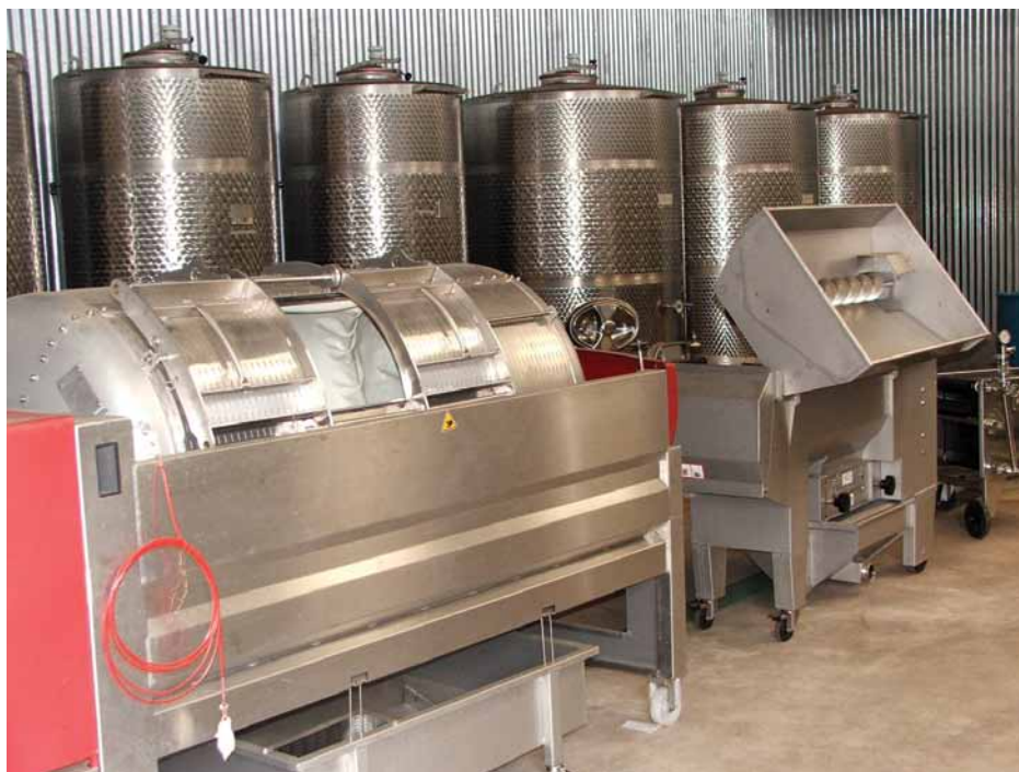
The stainless steel winemaking equipment is state of the art. The fermenters and aging tanks have cooling bands to control the temperature.
