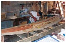
The bottom plank with the centerboard trunk stiffeners in place being screwed to the building platform by David Ramírez
