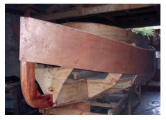
The first topsides plank, the cabin sides and part of the first bilge planks are fastened
