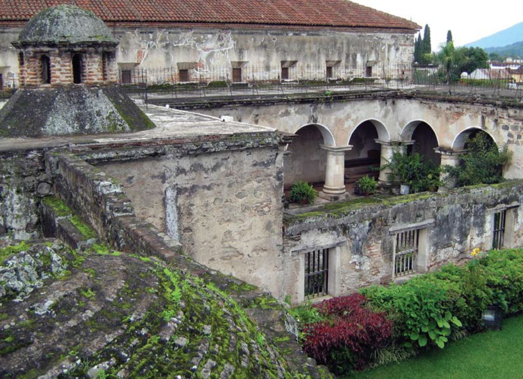
LEFT: Squat columns and arches of Capuchin cloister were designed for earthquake resistance ABOVE: Capuchin convent and gardens from above
