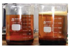
Biodiesel produced in a lab: top layer is biodiesel, bottom layer is glycerol
